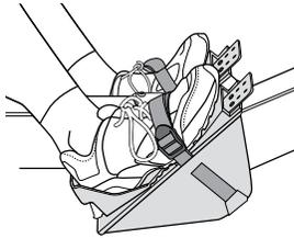
**Flexfoot:** Use the lowest setting (hole #1) for kids with the smallest feet. Very small feet may be even more comfortable with some foam placed below the heel. The goal is to have the footstrap crossing roughly over the ball of the foot.
